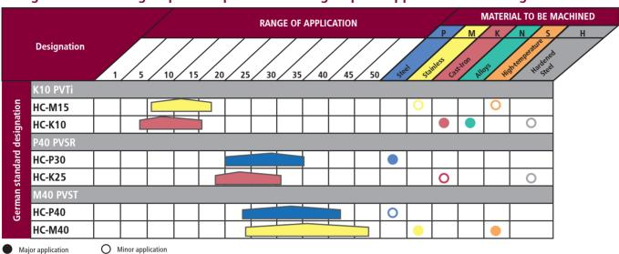
Full colour circle symbols represent: Major applications for materials to be machined. Hollow colour circle symbols represent: Minor applications for materials to be machined. The upper point of the pentagon-symbol indicates major applications. Sloping sides to the right or left indicate minor applications.
