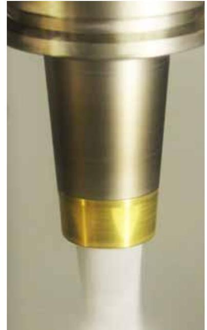
COOLCAP® in action: uniform, ring-shaped cooling jet
