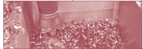
Up to our test, this has been machined with a Shell Type End Mill Body 52 310 (52 mm dia. r=6, z=5) and inserts 03 12 842K.
