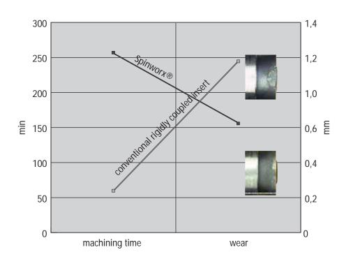
After a machining time of 265 minutes, we have identified a wear land of 0.63 mm for our Spinworx®-inserts. The end of cutting-edge life was still far away.
